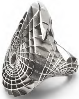
Crystal 82, ring, 2007, stellite, SLM (selective laser melting), hand polished
